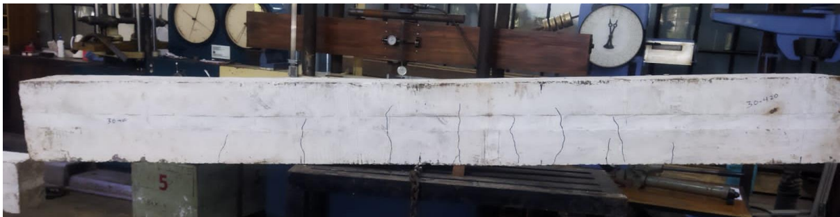
Figure 3.24: Cracks in beam reinforced with B420DWR and cast with 29.3 MPa concrete
