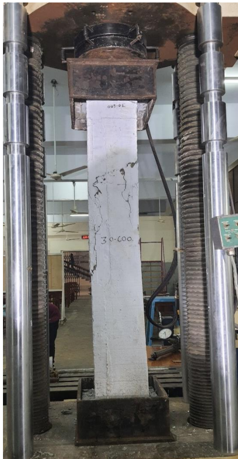
Figure 3.37: Failure patterns of column reinforced with B600C-R
