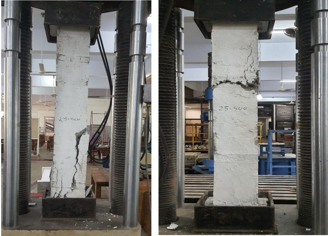
Figure 3.34: Failure patterns of column reinforced with (a) B420DWR (b) B500CWR
