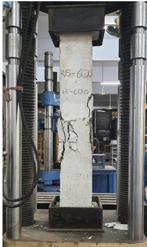
Figure 3.35: Failure patterns of column reinforced with B600C-R
