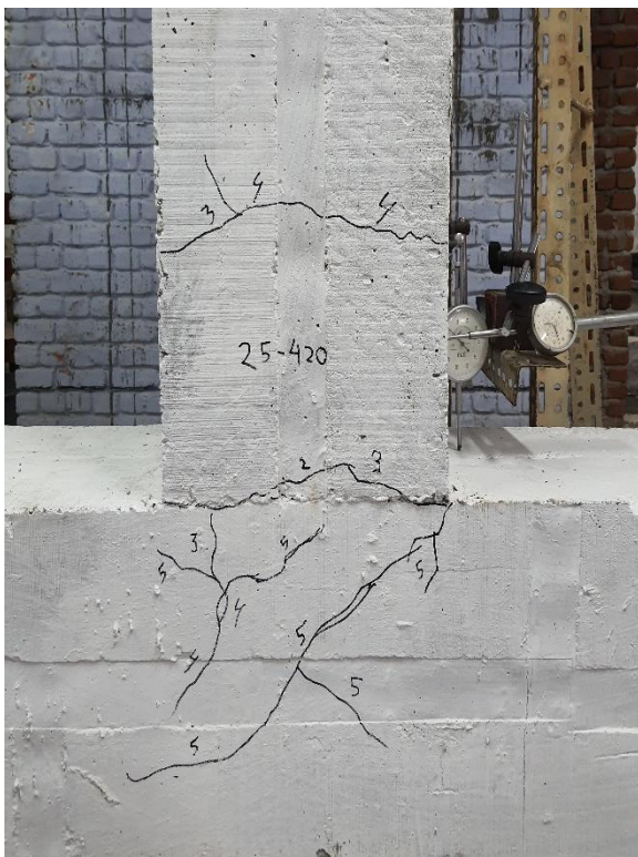
Figure 3.47: Cracking characteristics of joint reinforced with (a) B420DWR (b) B500CWR
