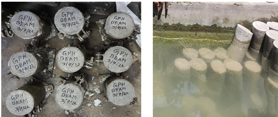
Figure 3.5: Cylinder Specimen Casting and Curing
