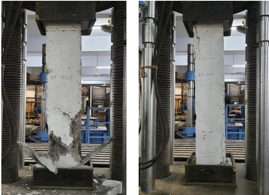
Figure 3.32: Failure patterns of column reinforced with (a) B420DWR (b) B500CWR
