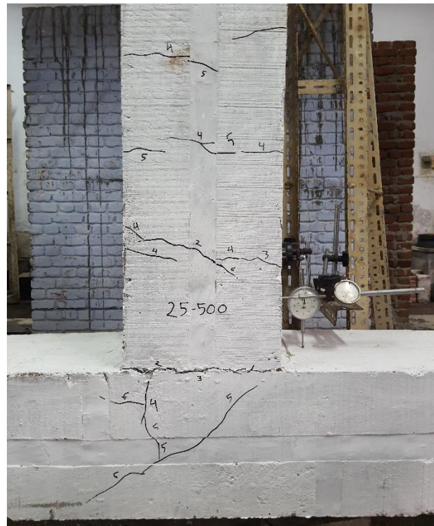
Figure 3.47: Cracking characteristics of joint reinforced with (a) B420DWR (b) B500CWR
