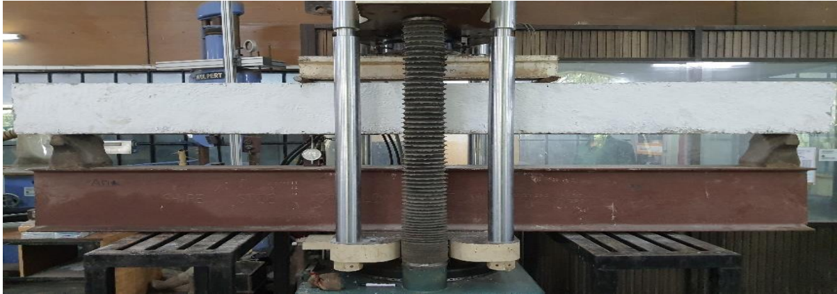
Figure 3.17: Two-point loading test setup of beam in laboratory
