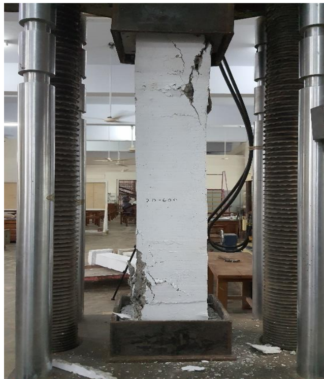
Figure 3.33: Failure patterns of column reinforced with B600C-R
