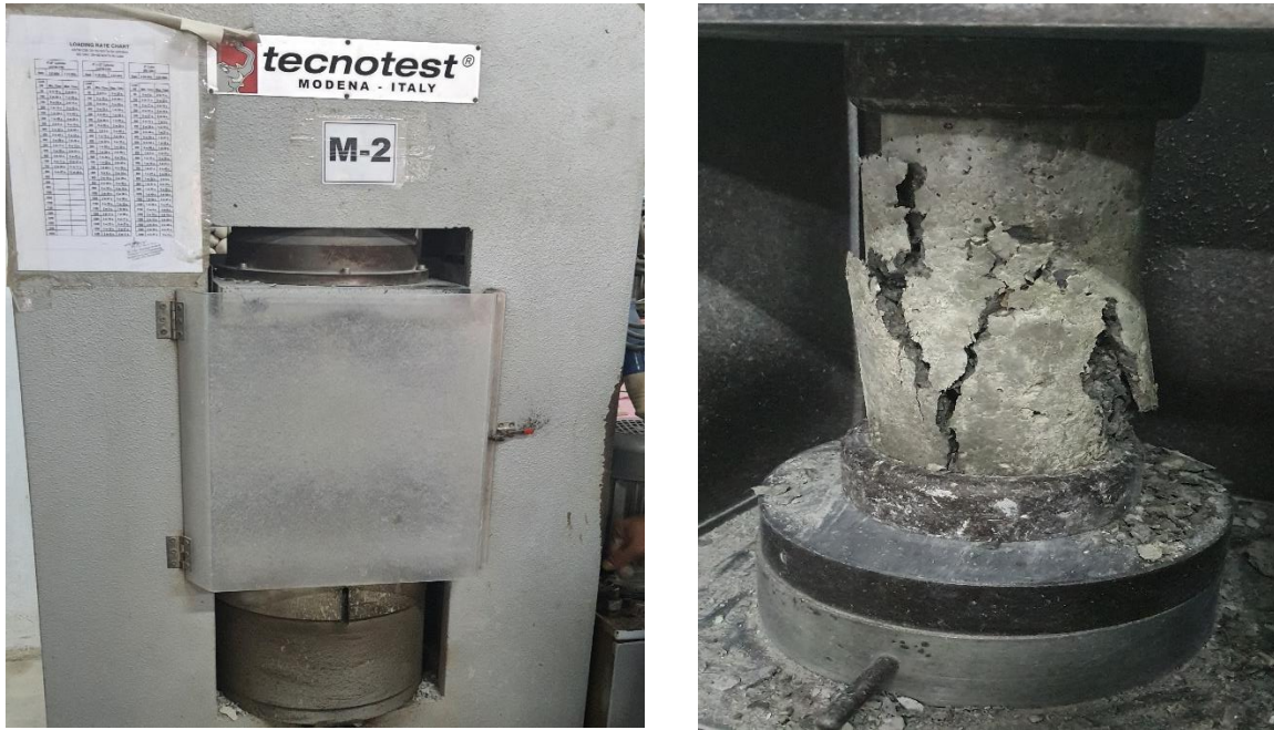
Figure 3.6: Compressive Strength test of Cylinder
