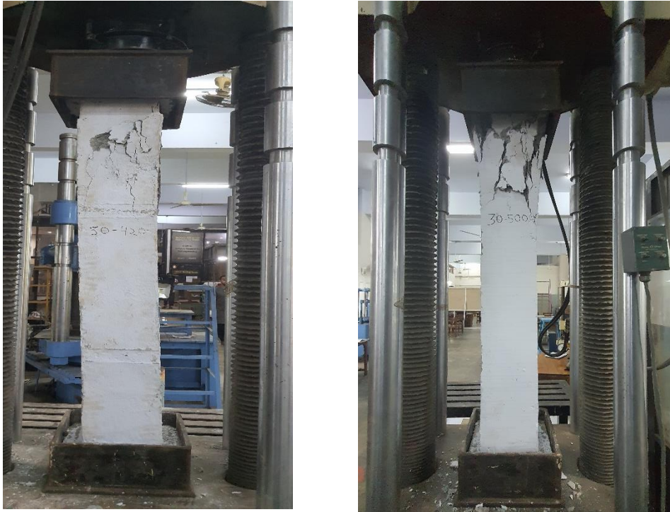
Figure 3.36: Failure patterns of column reinforced with (a) B420DWR (b) B500CWR
